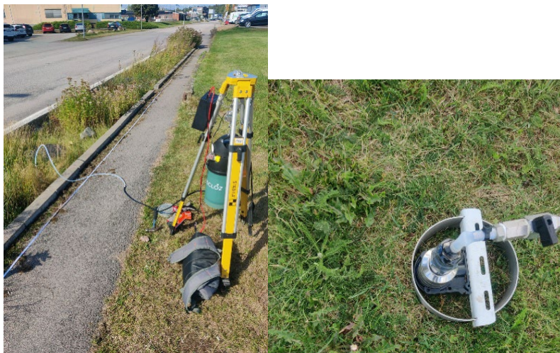
Figure 2. INFLOW infiltrometer prototype photos in field use in Växjö, Sweden
